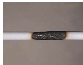
CPVC - After torch is removed
