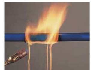
Other Plastics - initially when torch is applied
