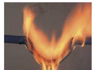
Other Plastics - After torch is removed
