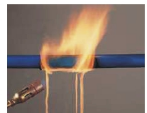
Other Plastics - initially when torch is applied
