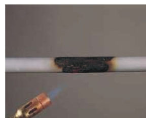
CPVC - initially when torch is applied
