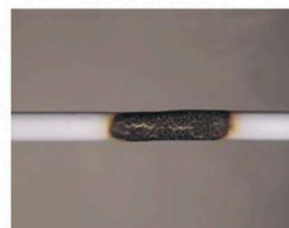
CPVC - After torch is removed
