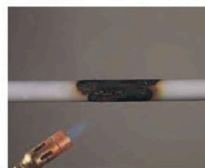
CPVC - initially when torch is applied
